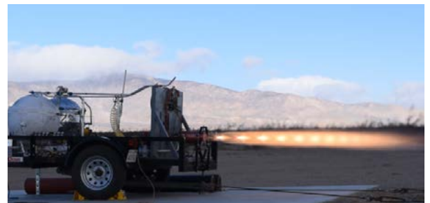
"Dropinator" dynamic test stand
